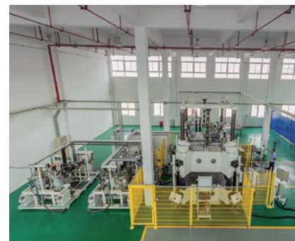
The MX mould carrier has a fixing area of 3,000 x 2,000 mm and a clamping force of 600 t.
