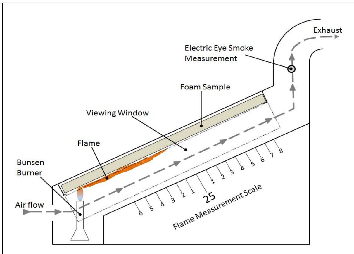
**Figure 3 – Diagram of Small Scale Burn Tunnel**
