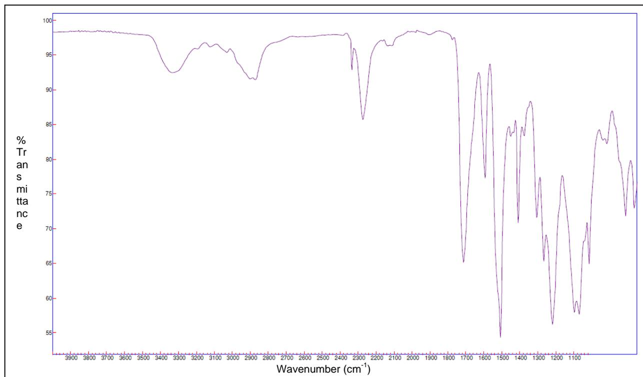
**Figure 6 – FTIR Spectrum of 14B10 Made with Surfactant 2**
