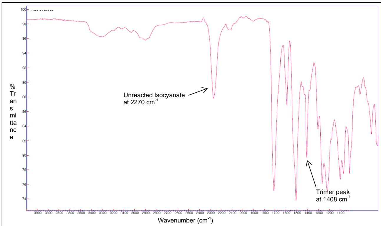
**Figure 5 – FTIR Spectrum of Cured Foam of 14B9 Made with Flame Retardant B**
