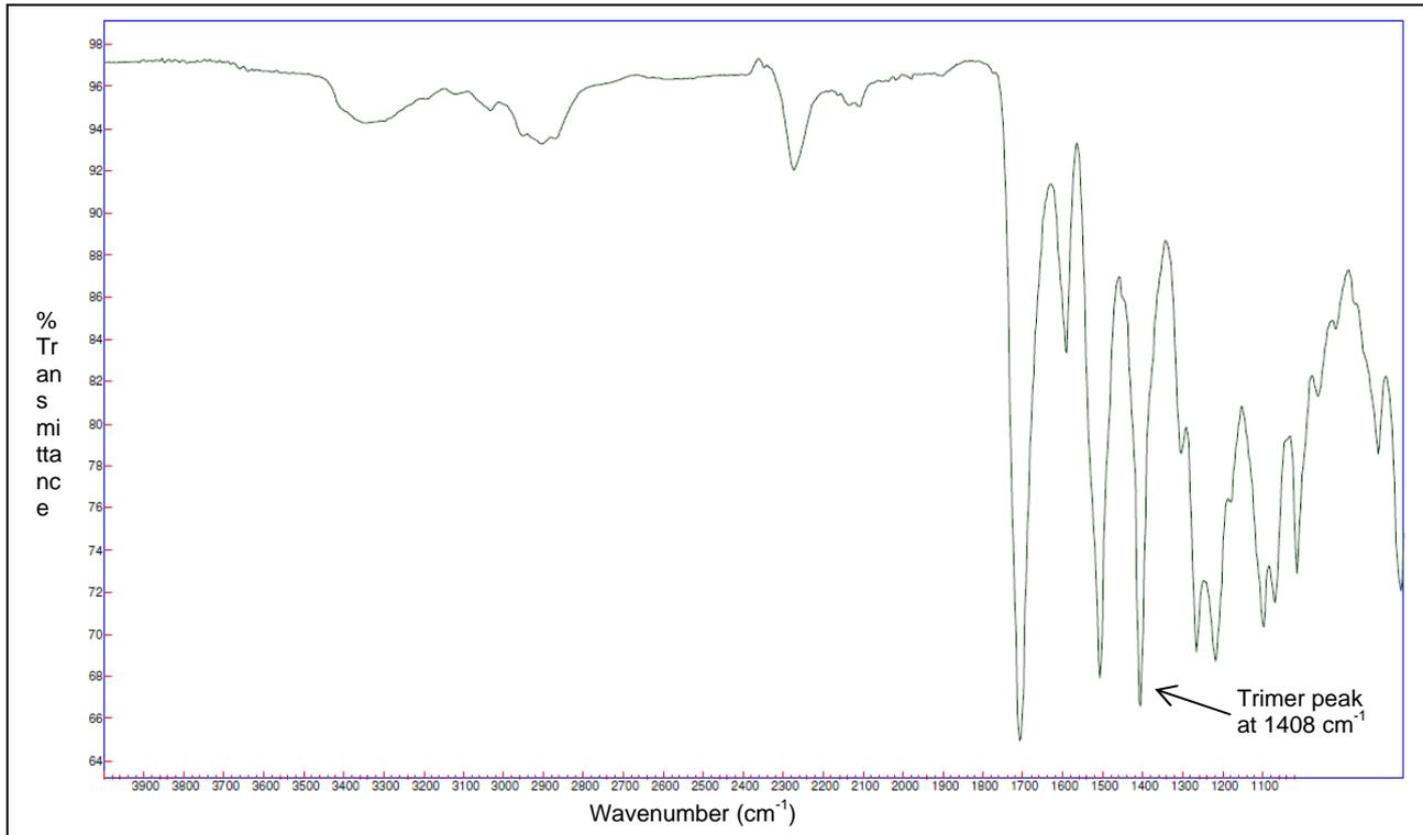
**Figure 4 – FTIR Spectrum of Cured Foam of 14B9 Control (Flame Retardant A)**
