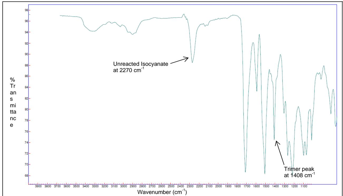
**Figure 5 – FTIR Spectrum of Cured Foam of 14B9 Made with Flame Retardant C**
