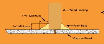
FoamNail® shown applied along the intersection of the gypsum and the lumber according to FSI application instructions.
