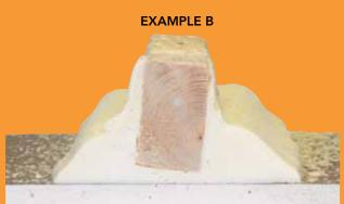
FoamNail® provides a strong adhesive bond when the lumber is straight and fits flush (Example A), and also fills in any gaps when the lumber is warped and cannot fit flush (Example B). (Note: Example A and Example B cross sections were cut from the same lumber/gypsum construction.)
